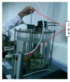
Connect flow meter with air tube and gas diffuser ball with the help of the transparent pipe.
